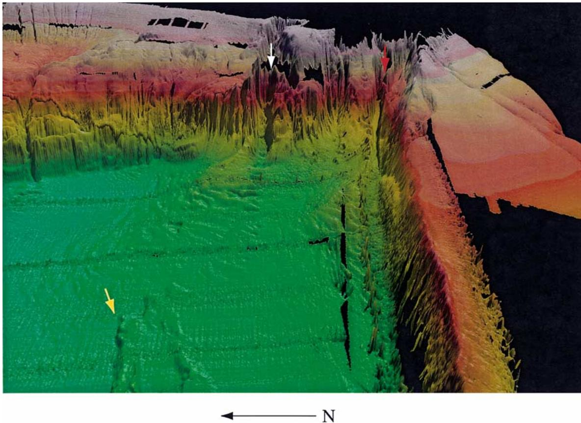
Figure 5. Three-dimensional perspective map of the Mendocino and Eel Canyons showing development of the proximal sediment fans at the mouths of the canyons. View azimuth is from the northwest. The two fans that formed at the bases of the Eel (white arrow) and Mendocino Canyons (red arrow) coalesce into one large fan extending several kilometers into the Gorda Plate abyssal plain. The northwest portion of the fan is offset by two large NE-SW trending scarps in the foreground (yellow arrow).
