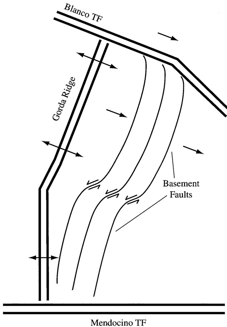
Figure 9. Line drawing of the structural interpretation for the deformation of the Gorda Plate based on offsets observed in the SeaBeam bathymetry presented. Left slip is observed in the southern section of the Gorda Plate, while the northern section appears to be moving passively with the Juan de Fuca Plate. Model is consistent with those proposed by Wilson (1989) and Stoddard (1987).
